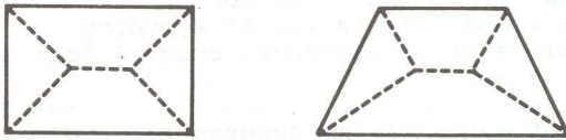
Fig. 2: Description of forms (rectangle and trapezoid) by the lines on which the centers of the maximal circles lie which can be inscribed into these forms.
