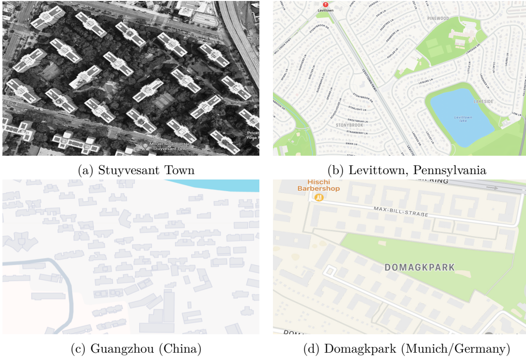
The figure shows the figure ground plans of four blocks that approximate the stylized chess block in Fig. (3a), and hence in turn benefit from an understanding of the generic chess block. The blocks “Stuyvesant Town” in New York and “Domagkpark” in Munich/Germany are centrally located, Levittown and Guangzhou are at their cities’ respective urban peripheries. Source: Google Earth/Google Maps.
