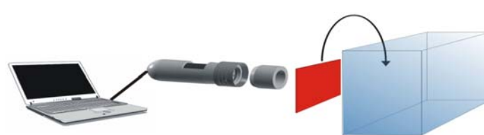
Schematic of the state of the art in imaging O 2 . Left: PC with software and for display. Center: Handheld portable instrument for lifetime imaging. Red film: Sensor membrane incorporating a quenchable luminescent probe for O 2 to be placed on the object of interest (a bioreactor, or skin, or an aircraft, etc.; symbolized by a cube)
