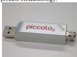
Optoelectronic system containing an RSB port (left) and a fiber connector (right) for fiber optic decay time-based sensing of \text{O}_2 .
