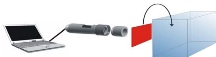
Schematic of the state of the art in imaging \text{O}_2 . Left: PC with software and for display. Center: Handheld portable instrument for lifetime imaging. Red film: Sensor membrane incorporated with a quenchable luminescent probe for \text{O}_2 to be placed on the object of interest (a bioreactor, or skin, or an aircraft, etc.; symbolized by a cube)
