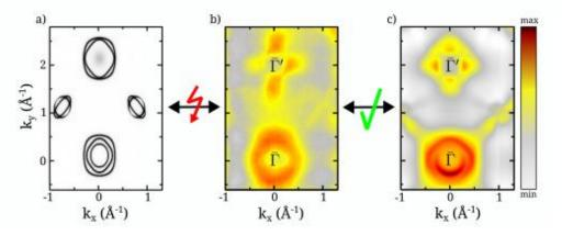
Fermi surface of the hightemperature superconductor Ba<sub>0.6</sub>K<sub>0.4</sub>Fe<sub>2</sub>As<sub>2</sub> as observed by ARPES (b) and modeled with (a) conventional ground-state theory and (c) advanced one-step photoemission modeling. (G. Derondeau et al. Sci. Rep. **7**, 8787, 2017)
