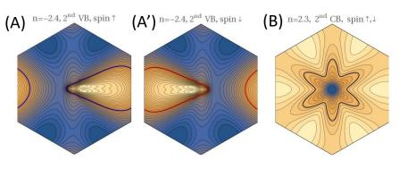
Energy contour maps showing the Fermi lines in the second valence band for (A) spin-up and (A') spindown electrons in the moiré Brillouin zone of TBG for filling fraction of 2.4 holes per moiré unit cell. Contiguous contour lines differ by a constant step of 0.02 meV, from lower energies in blue to higher energies in light color. (B) Energy contour maps showing the Fermi line in the second conduction band at filling fraction of 2.3 electrons per moiré unit cell.
