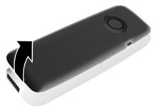
To **change the battery**, place your fingernail in the cavity in the casing and pull the battery upwards.
